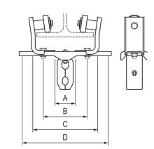
o Contact HARRINGTON when the Travel Beam width exceeds 6.9 inches (175 mm).
