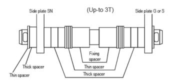
**Dimensions of Adjusting Collars** (Unit: mm)
