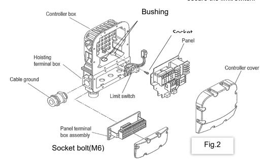
2. Disassembly to replace electrical components and cables in the connection box (common to hoists and trolleys)
