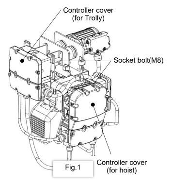
(1) Remove the socket bolts (For Hoist, Trolley 8 Pieces Each) from the controller cover and remove the controller cover.
