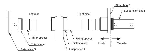
Adjusting spacer arrangement for Lug Suspension
