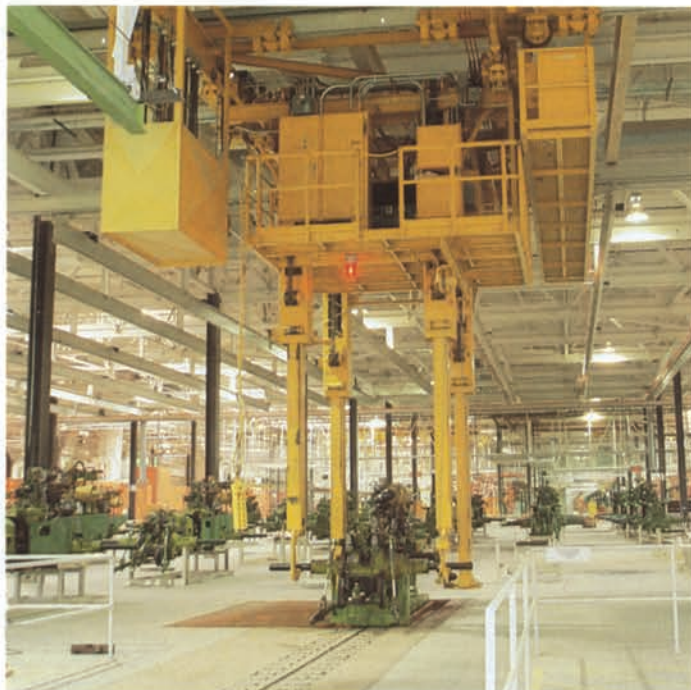
Chassis storage using horizontal automatic storage/retrieval system with two bridge cranes and chassis carriers.
