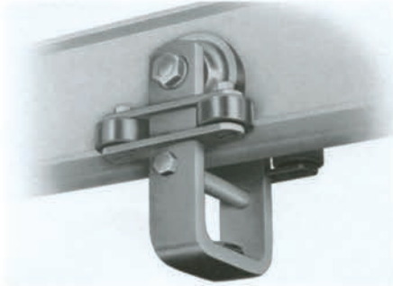
A two wheel trolley with flangeless wheels and guide roller is available to operate on a 2" and 3.33" flange application.
