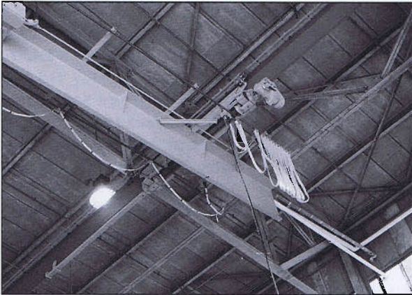
▲ Single girder 4-wheel end truck driven by a No. 2409 tractor drive.
