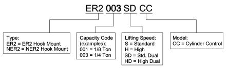
2.1.2 ER2 and NER2 Models - Harrington ER2 series hoist are available in two versions, the ER2 and NER2. These two versions are equipped with different options as standard equipment. The NER2 has a friction clutch mechanism that provides over winding protection. The ER2 has a mechanical load brake/friction clutch combination and an electronic count/hour meter in the control circuit. Refer to Figure 2-1 for the visual differences between the ER2 and NER2.
